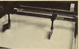
Above shows the increased wave at higher speeds compared with the preceding photograph. Below, waves form at the bump on the top of the liquid.
